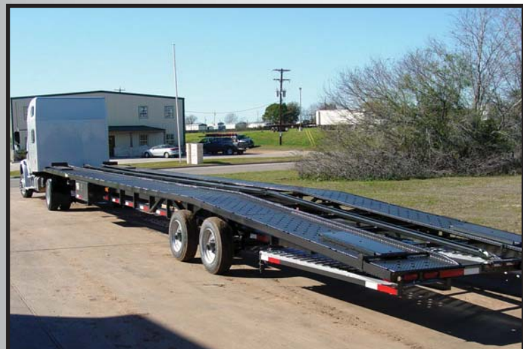
Trailer shown with dovetail break after axle and 10 K Super Single Tandems
