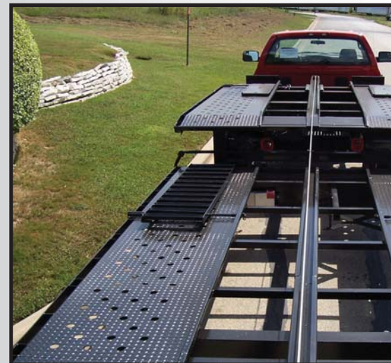
Unique tapered upper deck makes loading second tier safer and easier.
