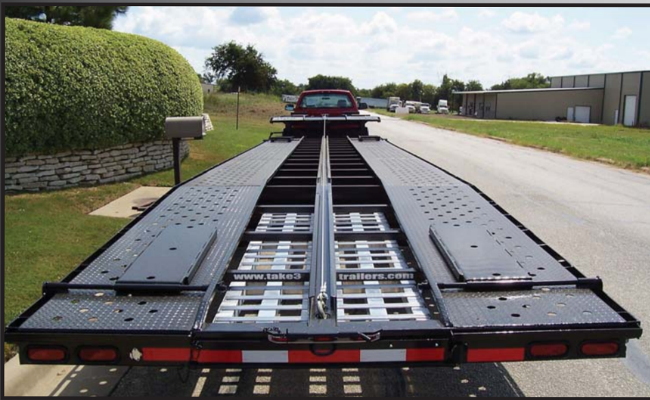
Standard 9' Aluminum Ramps with slide thru LOCKABLE ramp bumper cradles
